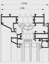
SlimLine 38 is a highly insulated system with inward and outward opening windows and doors, which combines elegance and comfort amidst a unique design. SL 38 is available in two different minimalistic design variants, Classic and Cubic, to perfectly match the architectural aspect of the building. The windows and doors can accommodate double and triple glazing without losing the ultra-slim look.
